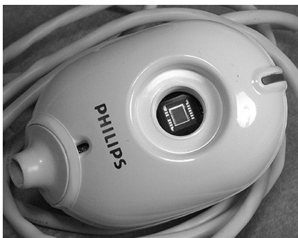
FIGURE 51. CCD image sensor (in webcam with lens removed)
