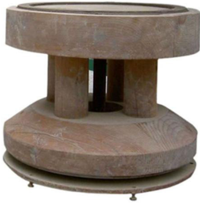
Picture 8: Wooden Kick Wheel Used in S. Korea. Picture 9: Metal Kick Wheel Used in S. Korea.
