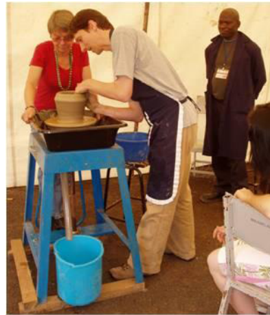
Picture 12: Treadle Wheel Used in Kenya
